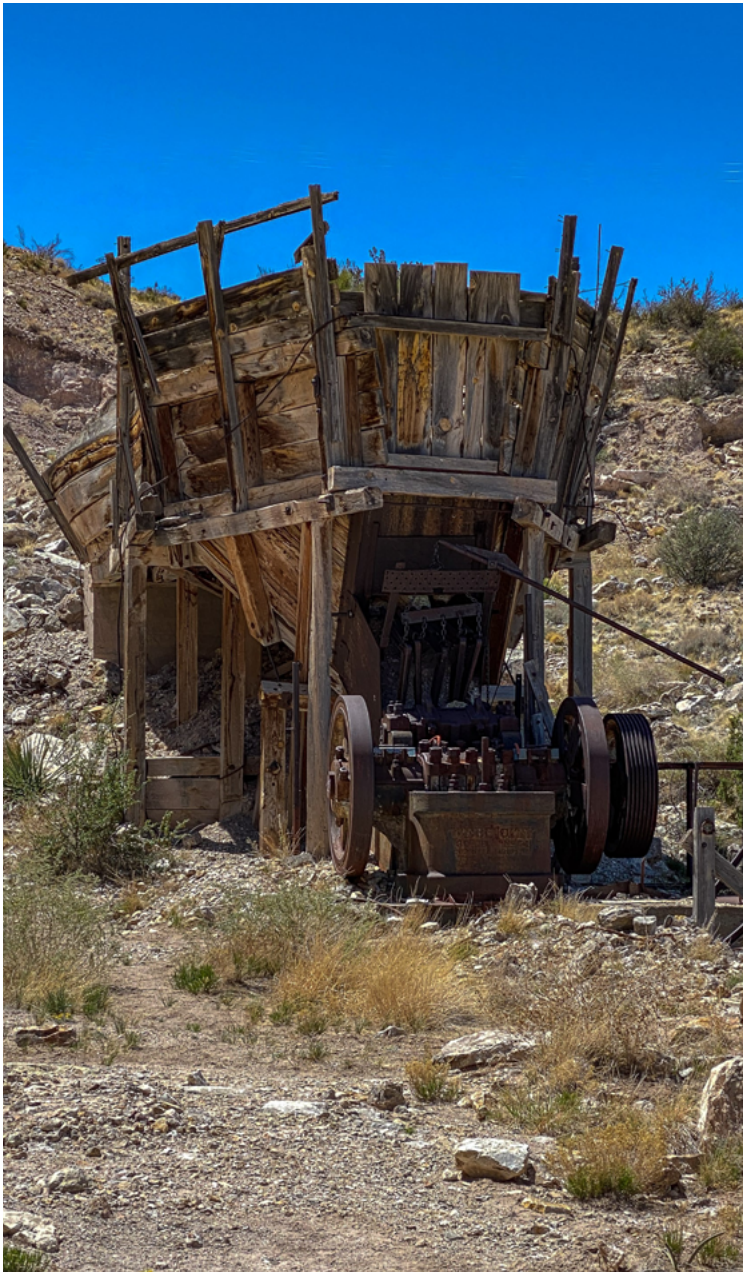
Small historic stamp mill at Blanchard lower with ore bin still full (BW)
